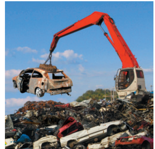
Figure 15.3: Powerful magnets are used to lift discarded cars in a junkyard.
